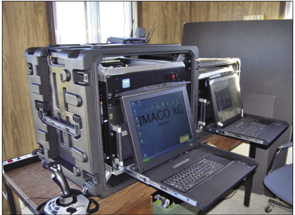
The rack-mounted PC units house the tracking PC and GUI, and the mission record and analysis system (above).
