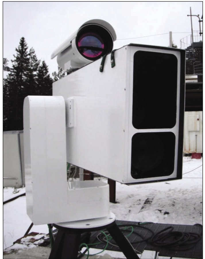
The camera enclosure contains digital tracking cameras as well as a high-speed camera (above). The IR camera is shown on top of the camera enclosure and the entire payload is mounted over the centre of rotation to eliminate off-axis parallax errors.
