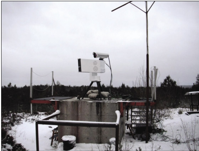
The IMAGO Tracking System is installed on the pre-surveyed location (above). The tracking system allows for input of survey data in both Cartesian NEU or WGS84 formats.
